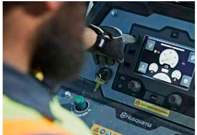
The robust digital display enables precise control of functions such as the optional electronic tracking system (ETRK) which assists in cutting a straight line.
